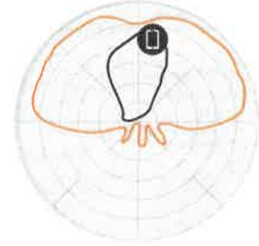
Figure 5 - T310d 5GHz Elevation Antenna Patterns
